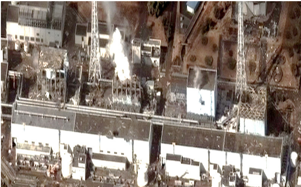
Fig. 11 Nuclear power plant explosion due to disorder of cooling system caused by Tsunami.
